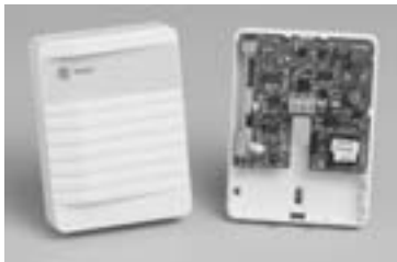
Figure 47. CO 2 wall sensor
